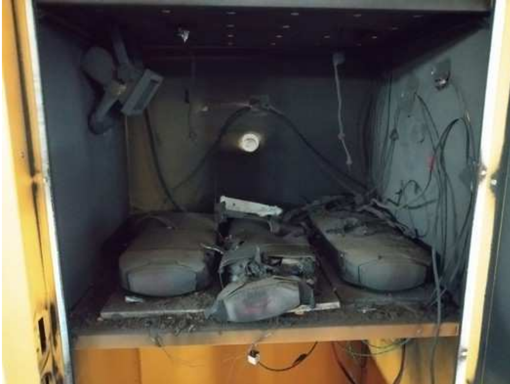
f4.3 Situation inside the ONOS Charge Safe after the test
