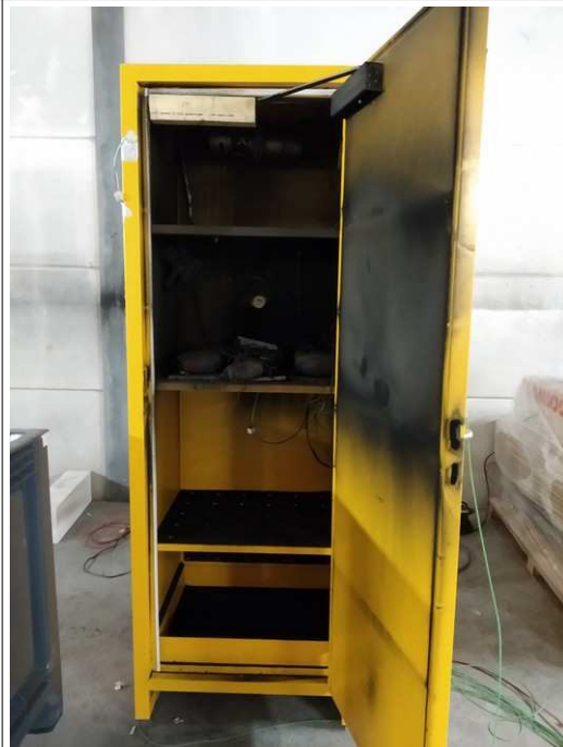
Inside of the ONOS Charge Safe after test
