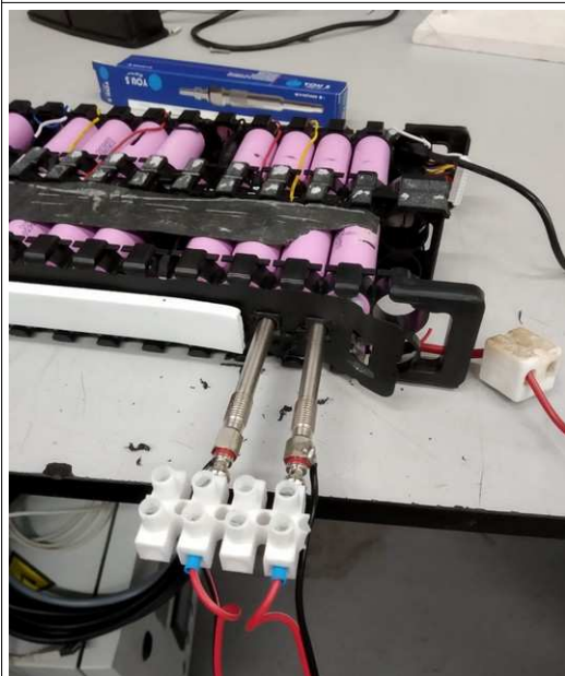
Prepared battery with glow plug
